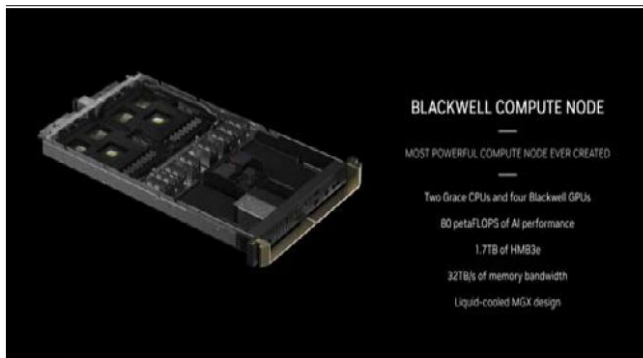
Figure 9: A Blackwell compute node consists of two CPUs and four GPUs
