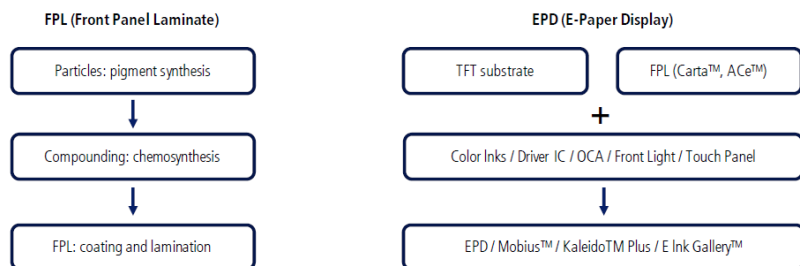
Figure 12: Production process for EPD
